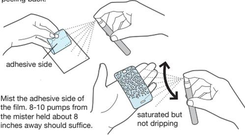
Mist the adhesive side of the film. 8-10 pumps from the mister held about 8 inches away should suffice.
